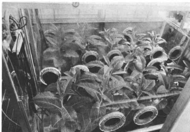
Figure 2. Automated culture of isotopically enriched plants in a closed growth system
